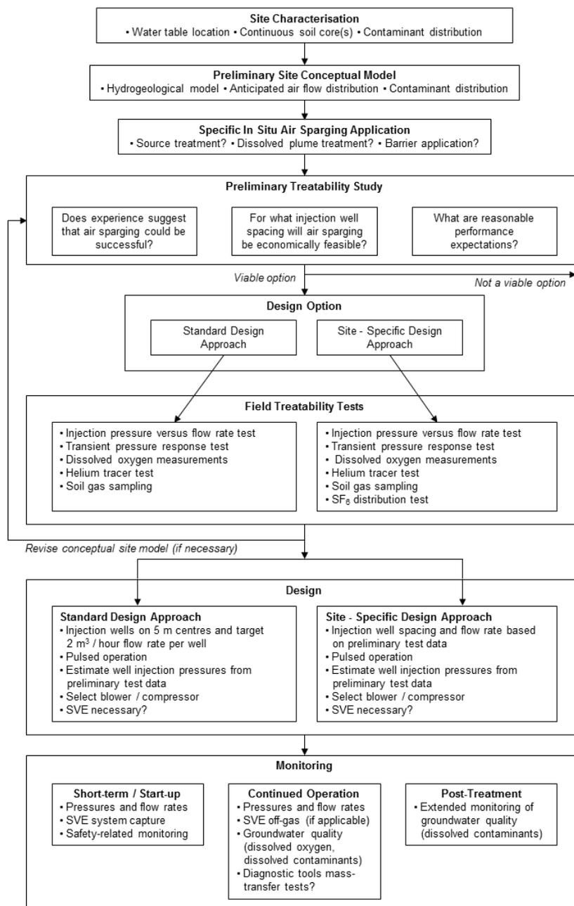
Figure 2: Sequence of activities during implementation of air sparging, from Leeson et al (2002)
