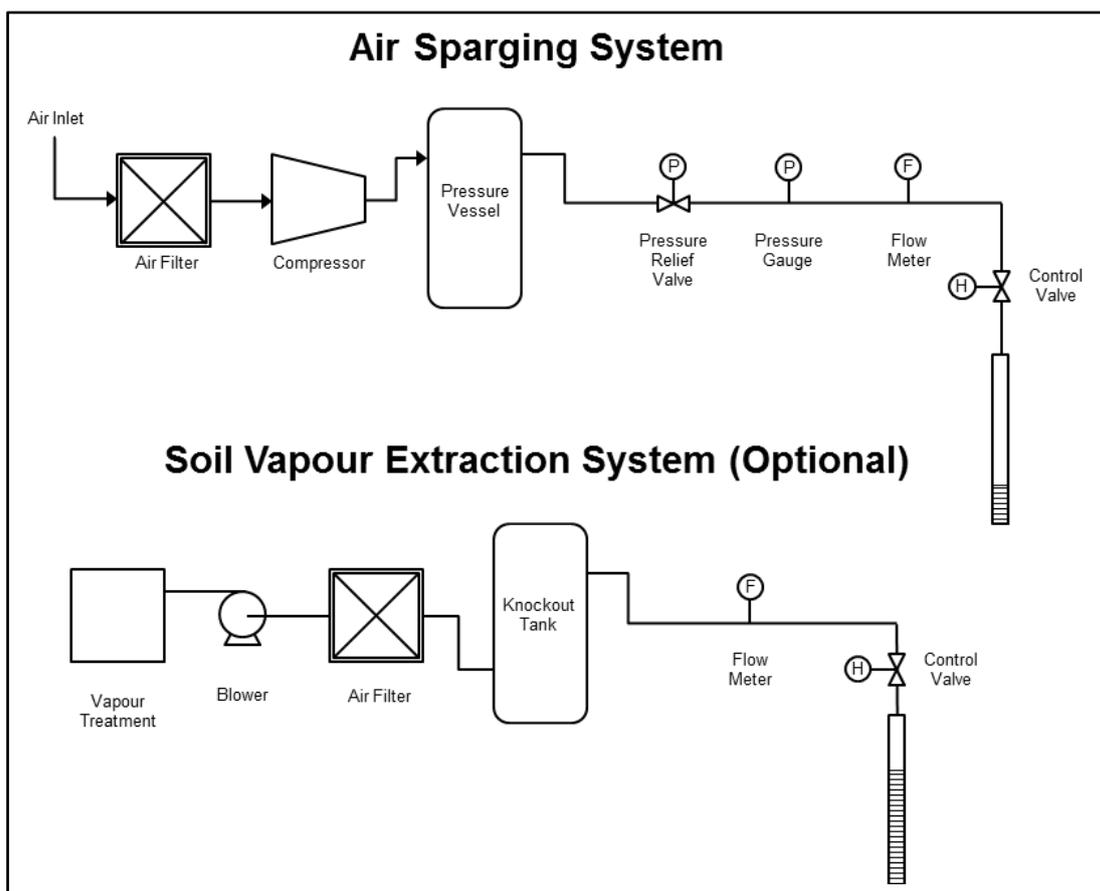
**Figure 5** Components of a typical air sparging system, with SVE control system, from NAVFAC (2001)
