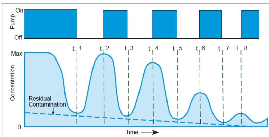
**Figure 5: Schematic illustrating the pulsed pumping concept**
