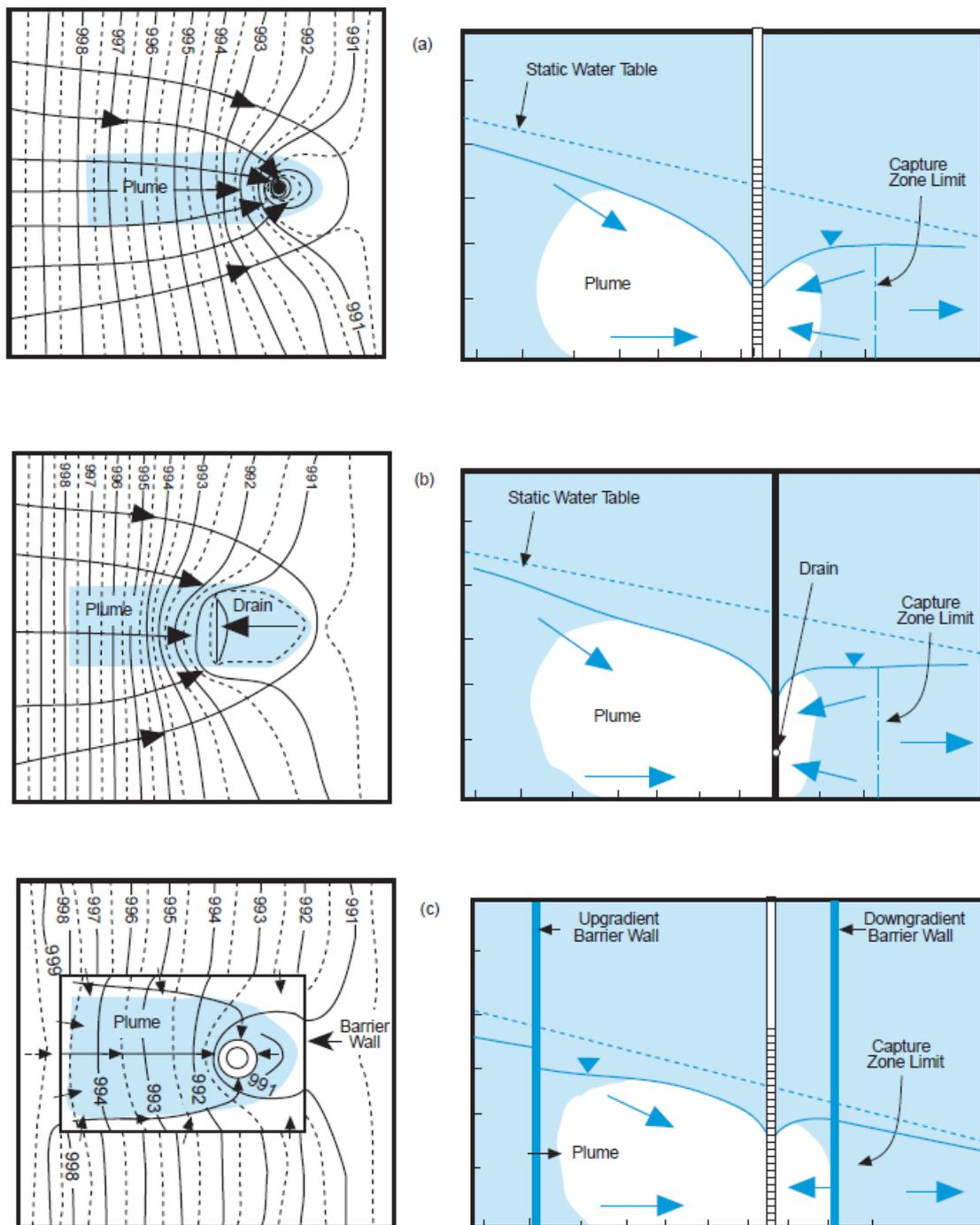
Figure 1 Examples of hydraulic containment from US EPA (2002)
