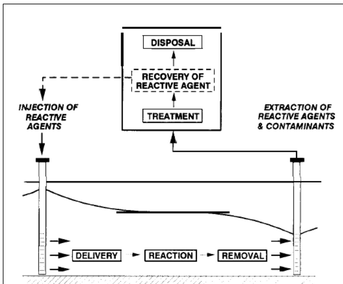
Figure 2: Schematic of using chemical enhancement to supplement P&T systems
