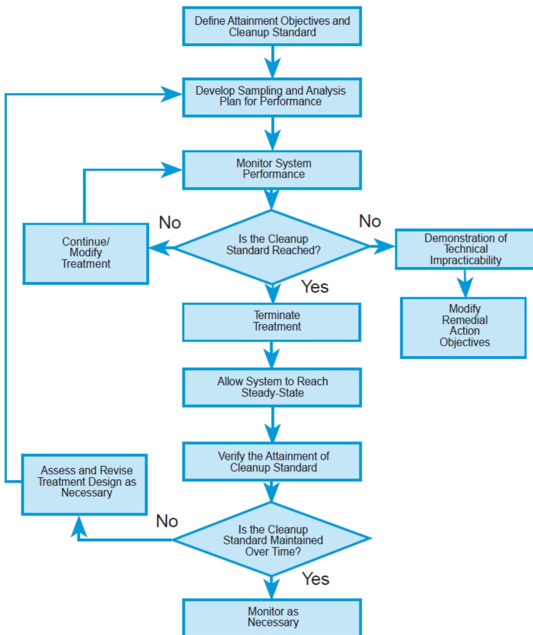
**Figure 6: Flow chart to predict the success and/or timeliness of closure of a P&T system**
