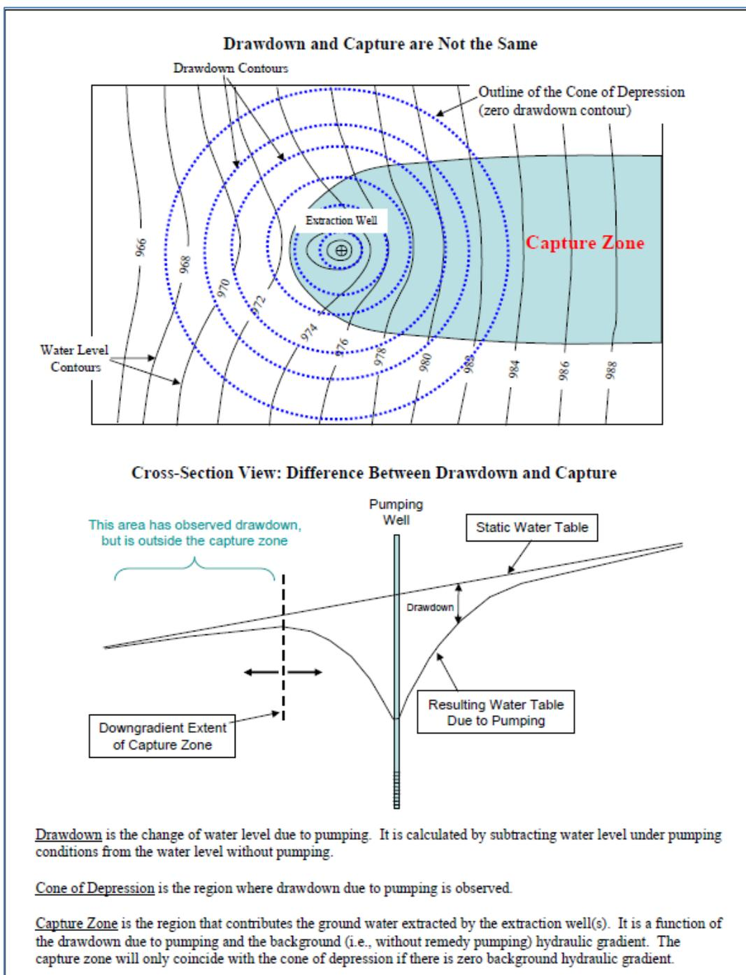
Figure 4: Schematic illustrating the difference between drawdown and capture
