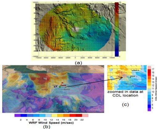
Figure 5 (a) CDL generated wind map on a terrain following layer at hub height (b) Comparison of CDL scan with the model generated wind map (b) arrows represent CDL wind direction coloured as wind speed magnitude while base represent WRF wind speed magnitude with wind barbs
