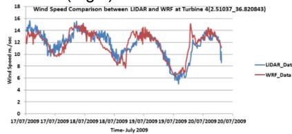
Figure 4 Comparison of wind speed between CDL and WRF predicted wind at 45 m (10 mins sampling) from 17 to 20 July 2009 (Time in UTC)
