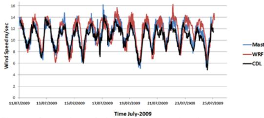
Figure 3 Comparison of wind speed comparison between mast A (10 mins sampling), WRF predicted wind (10 mins sampling) and CDL at 39 m height (Time UTC)
