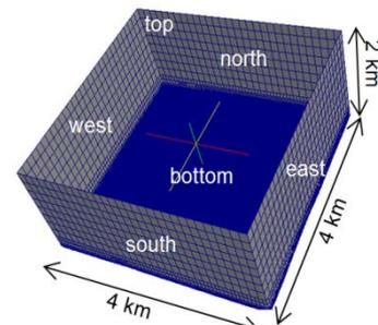
Figure 6 OpenFOAM domain and mesh with specified patches
